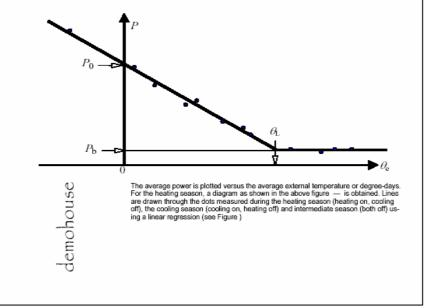
Energy Signature techniques are used to calculate the dynamics of each building and its relative performance against the local climate.
